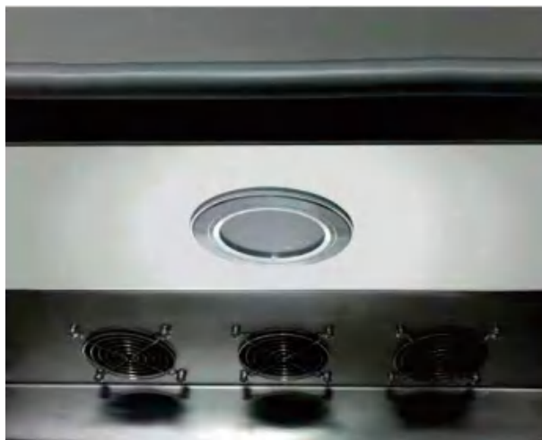
Automatic exhaust system on top of working cabin
